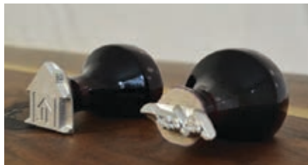
Magnesium dies mounted on wood handles
