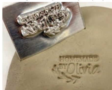
Magnesium mounted on aluminum block
