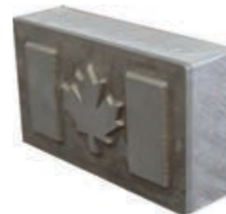
Magnesium mounted on aluminum block
